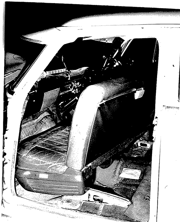
Fig. 10.17 Front seat completely off adjustment runners, 1953 Ford Customline.
