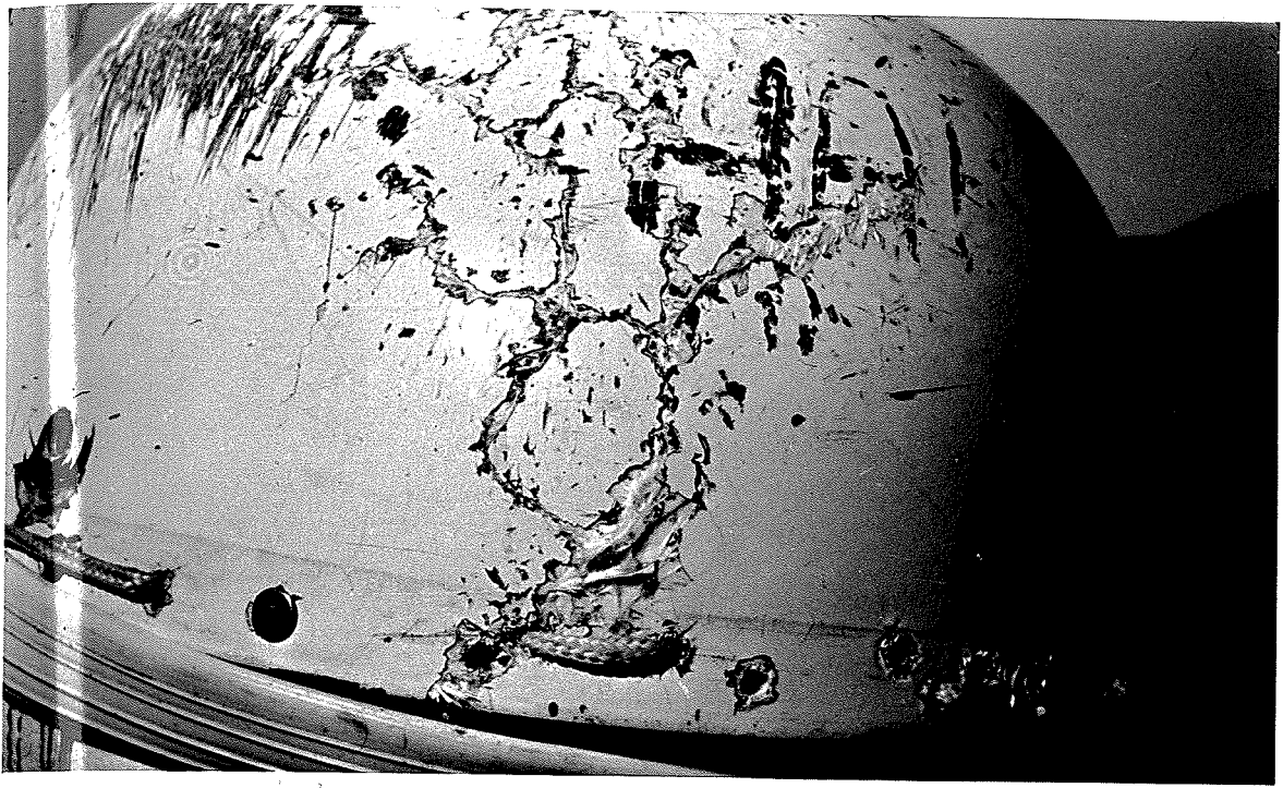
Fig. 6.14 Note fracture lines in shell of helmet.
