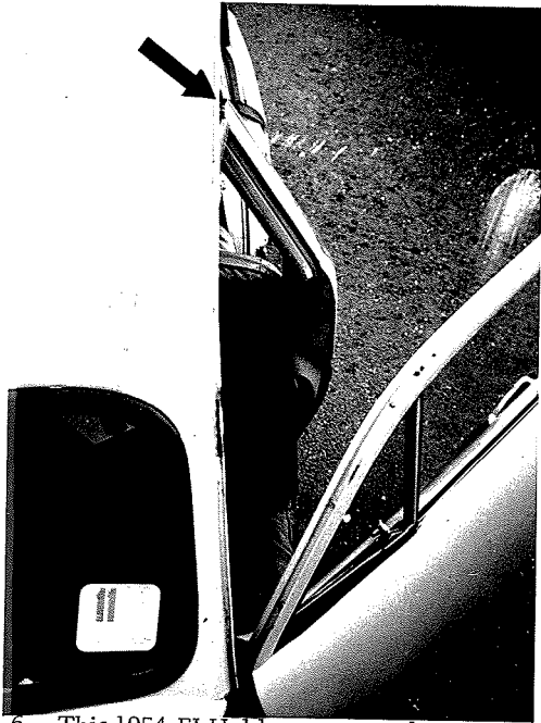
Fig. 12.6 - This 1954 FJ Holden was struck on the right side by another car. The front seat transmitted the force of the impact across the car to the centrepost, which was pushed out as shown, the spot welds being partly torn away (arrow). The rear door had been removed previously.
