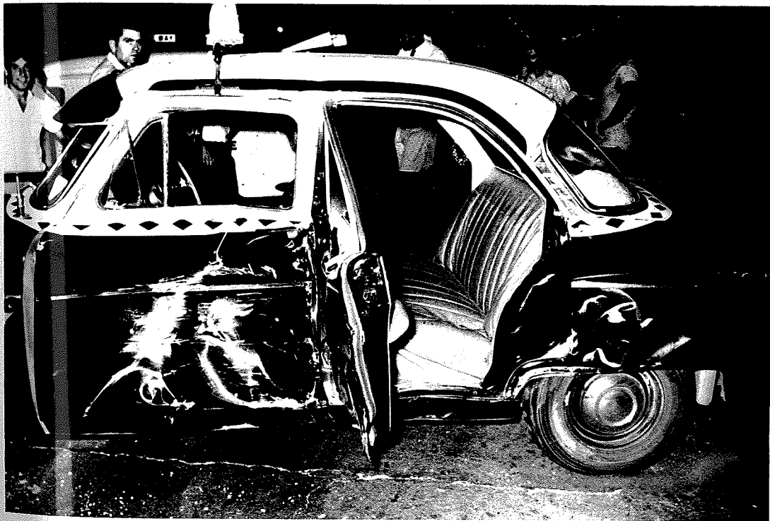
Fig. 8.4 1959 Ford Zephyr, struck by the Peugeot shown in Figure 8.3. Note that the rear door has come open.
