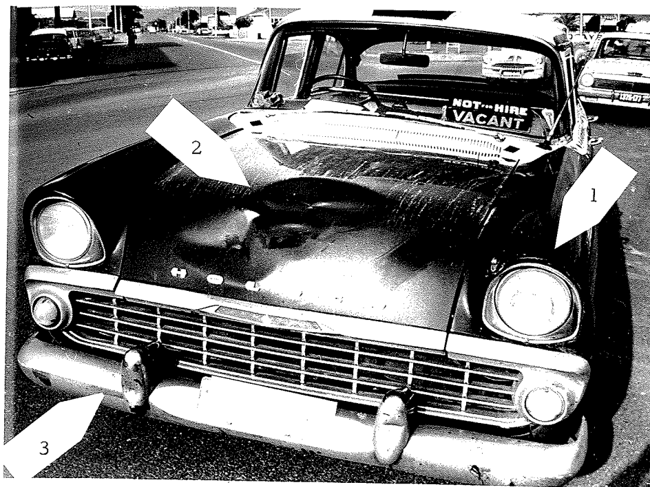
Fig. 5.10 Case 0160: impact of front of car with side of bicycle. Arrows indicate marks made by (1) handlebar on left headlight of car, (2) the seat of the bicycle and the rider's hip on the top of the bonnet, (3) the rear axle of the bicycle on the right bumper overrider.
