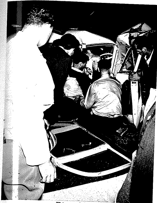
Fig. 10.16 Driver trapped in an FX Holden by the front seat, which moved forward in the collision.
