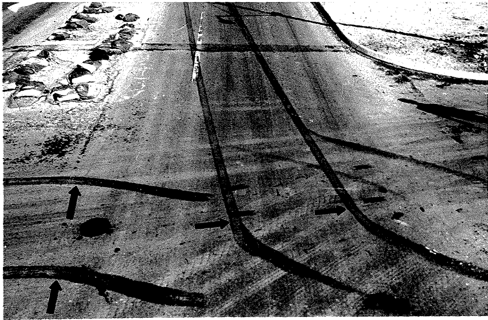
Fig. 13.11 Collision between a bus and a car. The arrows indicate the positions of the front wheels on impact.
