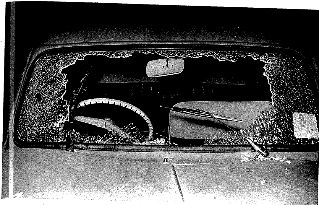
Fig. 11.7 1958 Simca windscreen, struck by passenger's head. (See also Fig. 11.5 for fragments from this screen.)
