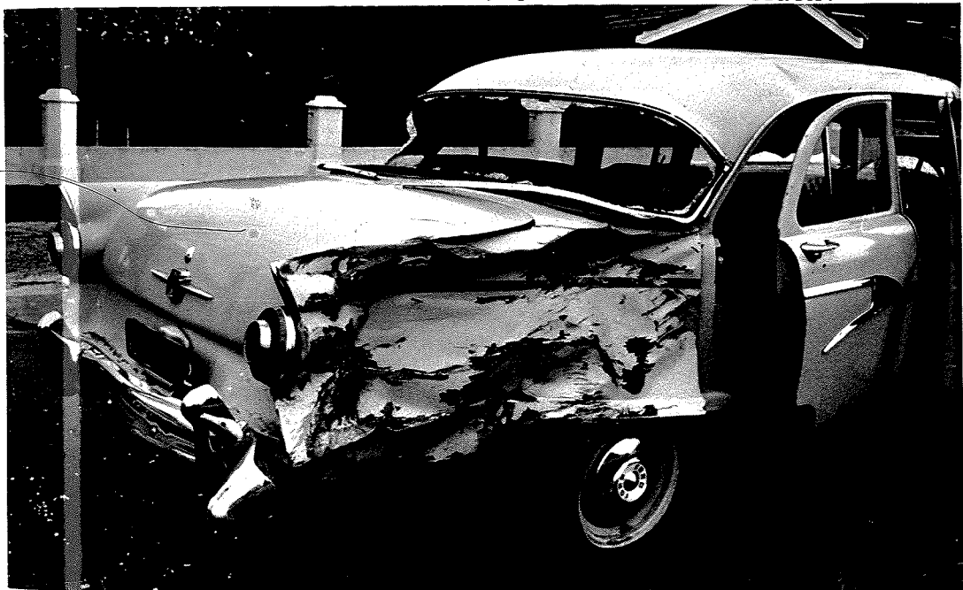
Fig. 8.26 The doors of this Ford Customline came open during the accident shown in Figure 8.28.
