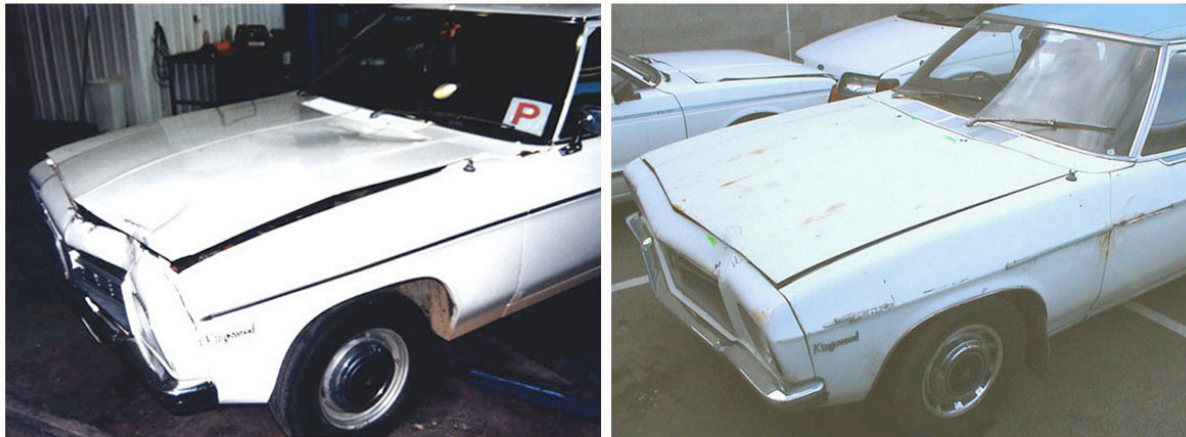
Figure 13-4 The accident damage from the impact (left) and the damage produced in the physical reconstruction (right) of case PED057-99.
