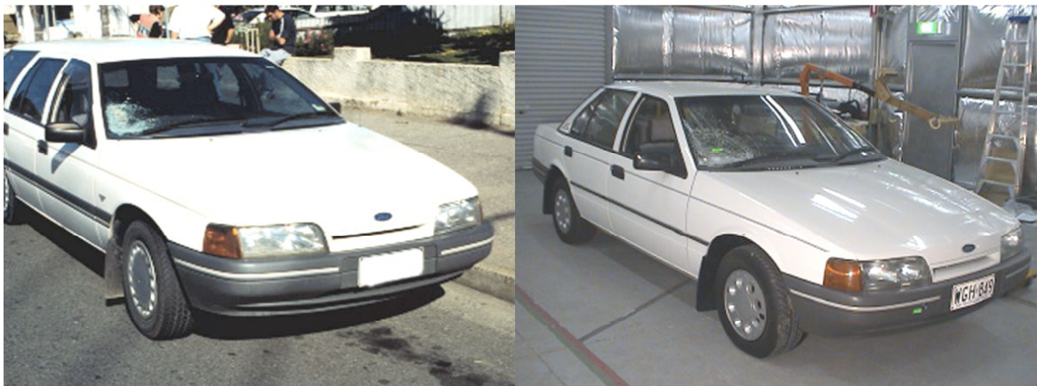
Figure 9-4 A general view of the accident damage (left) and the damage produced by the reconstruction (right) of the head and leg impacts in case PED035-99.
