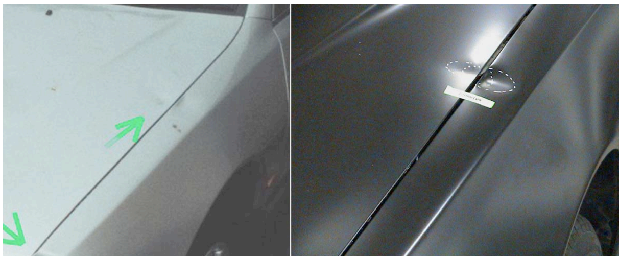
Figure 14-6 Close-up of the damage caused by impact with the child pedestrian's head (left) and the damage produced in the reconstruction (right) of case PED061-99.
