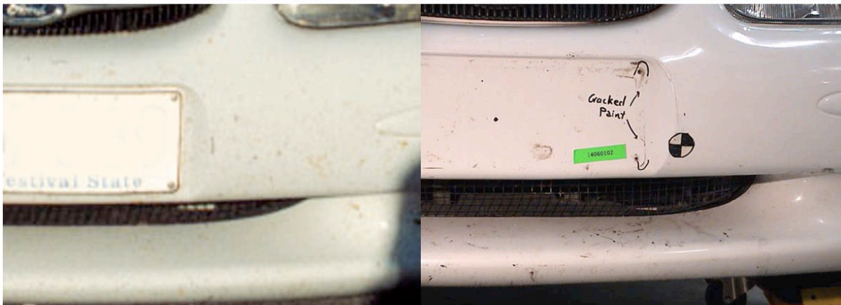
Figure 11-9 Knee shear displacement recorded for the physical reconstruction of case PED049-99.
