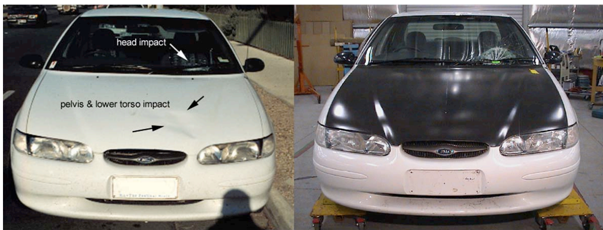
Figure 11-4 A general view of the accident damage (left) and the damage produced by the reconstruction (right) of case PED049-99.
