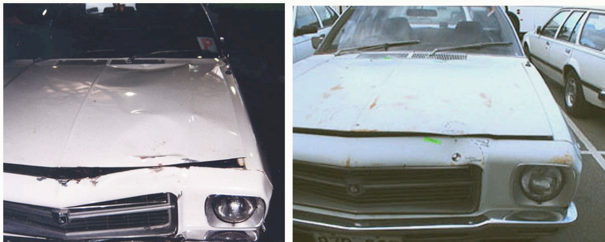
Figure 13-9 A close up front view of the accident damage from impact with the pelvic area (left) and the damage from the reconstruction with the Upper Legform (right) of case PED057-99.
