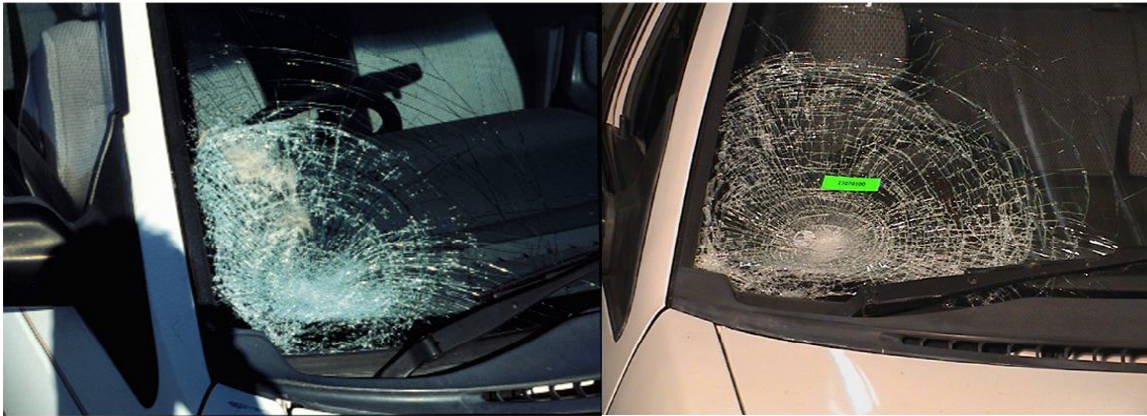
Figure 9-6 A front close up view of the vehicle involved, showing where the head impact occurred (left) and the damage as produced by the reconstruction (right) of case PED035-99.
