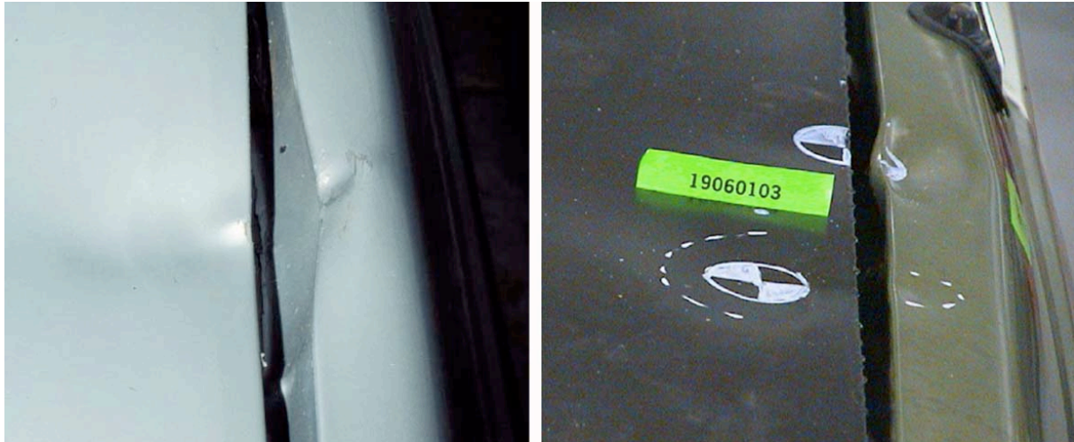
Figure 7-8 Damage caused by impact with the pedestrian's head (left) and the damage produced in the second reconstruction (right) of case PED011-99 (test 19060103).
