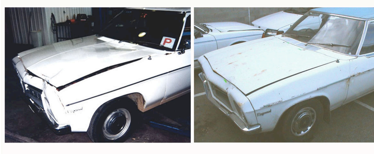
Figure 4-2 The deformation of the bonnet caused in the collision in Case PED057-99 (left). The deformation caused by the reconstruction tests was much less (right). The deformation created in the collision may have protected the head of the pedestrian by lifting the bonnet surface away from the under bonnet components of the car.
