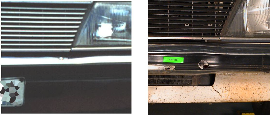
Figure 12-10 Close-up view of the vehicle involved in the actual pedestrian impact compared with the reconstruction of case PED056-99, very minor denting on the steel bumper bar in both cases.
