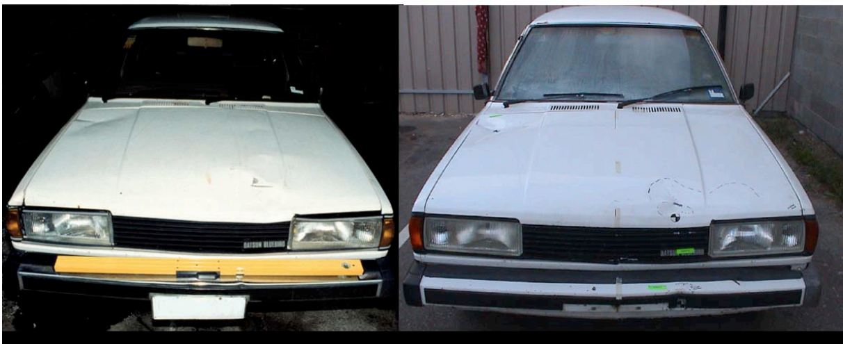
Figure 8-4 A general view of the accident damage from the impact (left) and the damage produced in the physical reconstruction (right) of case PED018-99.
