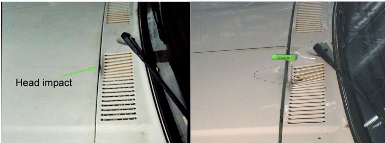
Figure 8-6 A side view of the damage caused by impact with the pedestrian's head (left) and the damage produced in the reconstruction (right) of case PED018-99.
