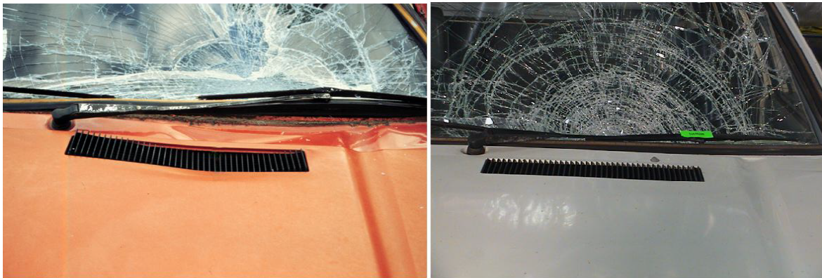
Figure 12-6 The accident damage caused by the impact with the head of the pedestrian ( left ) and the physical reconstruction damage of the head impact ( right ) in case PED056-99.
