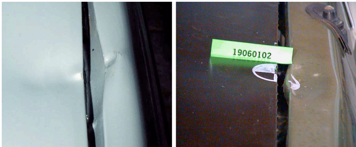
Figure 7-6 Damage caused by impact with the pedestrian's head (left) and the damage produced in the reconstruction (right) of case PED011-99 (test 19060102).
