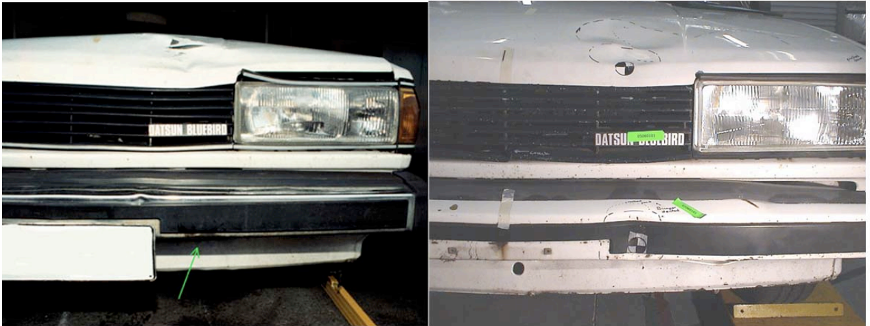
Figure 8-12 A close up front view of the accident damage from impact with the pelvic area (left) and the damage from the reconstruction with the Upper Legform (right) of case PED018-99.
