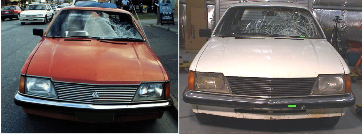
Figure 12-4 A general view of the accident damage (left) and the damage produced by the reconstruction (right) of case PED056-99.
