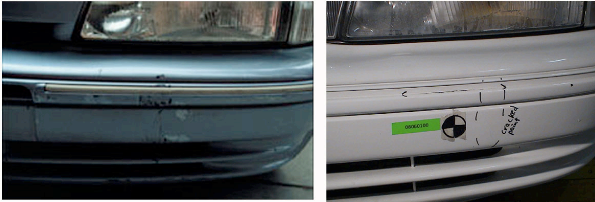
Figure 15-9 Close up front view showing the accident damage to the bumper (left) and the damage produced by the reconstruction (right) with the Legform of case PED064-00.
