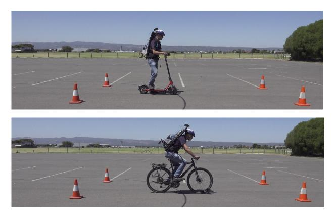
Figure 5.2 Testing the e-scooter and bicycle braking performance.
