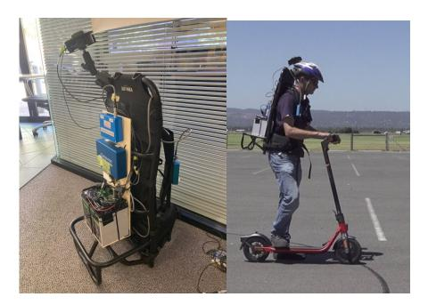
Figure 5.1 (a) Instrumented backpack (b) Instrumented backpack fitted to e-scooter rider.
