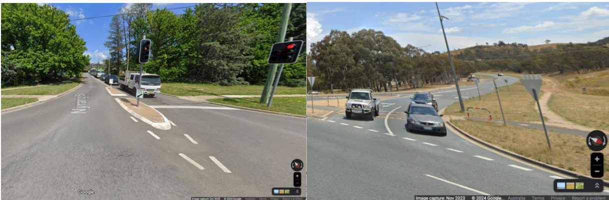
Figure 3.9 (a) Crossing point with insufficient protective space in the median (b) Crossing point with insufficient opportunities to cross.
