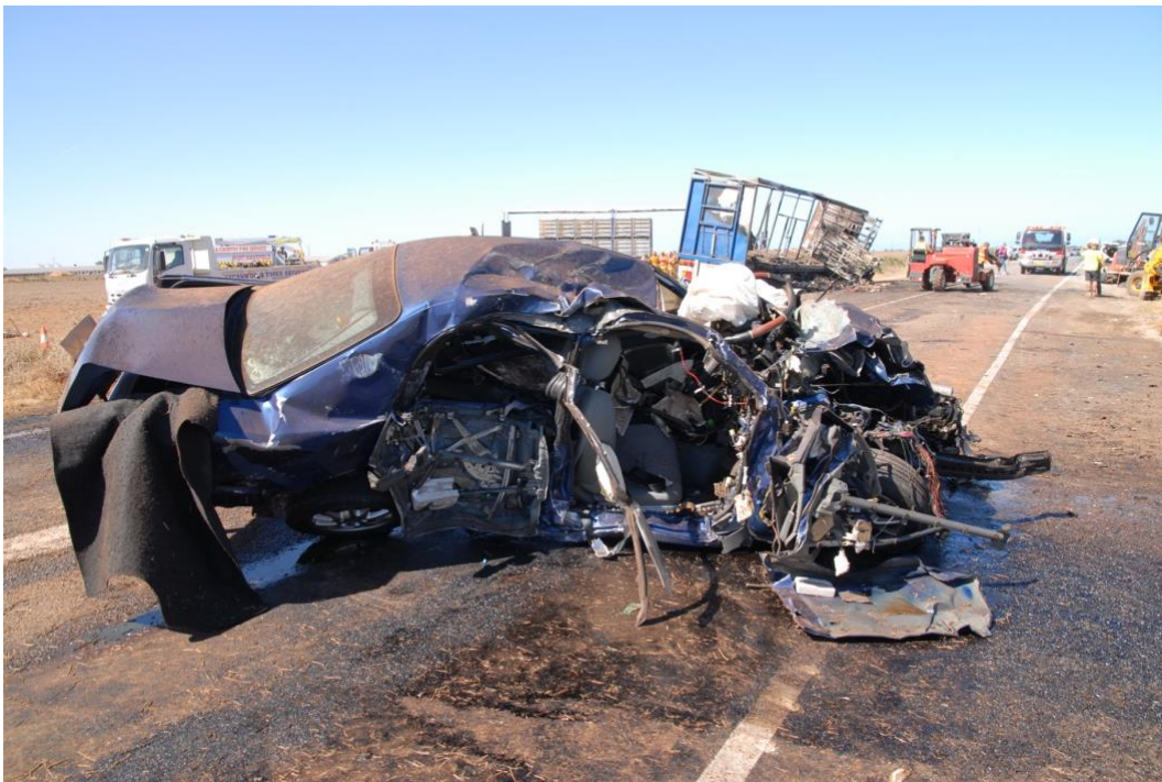
Figure 3.11 The massive amount of damage inflicted upon a light vehicle in a head on crash with a truck
