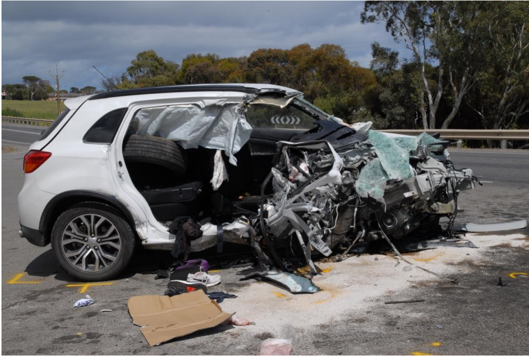
Figure 3.6 Typical damage suffered in a drift into oncoming lane head on crash on a high-speed road.
