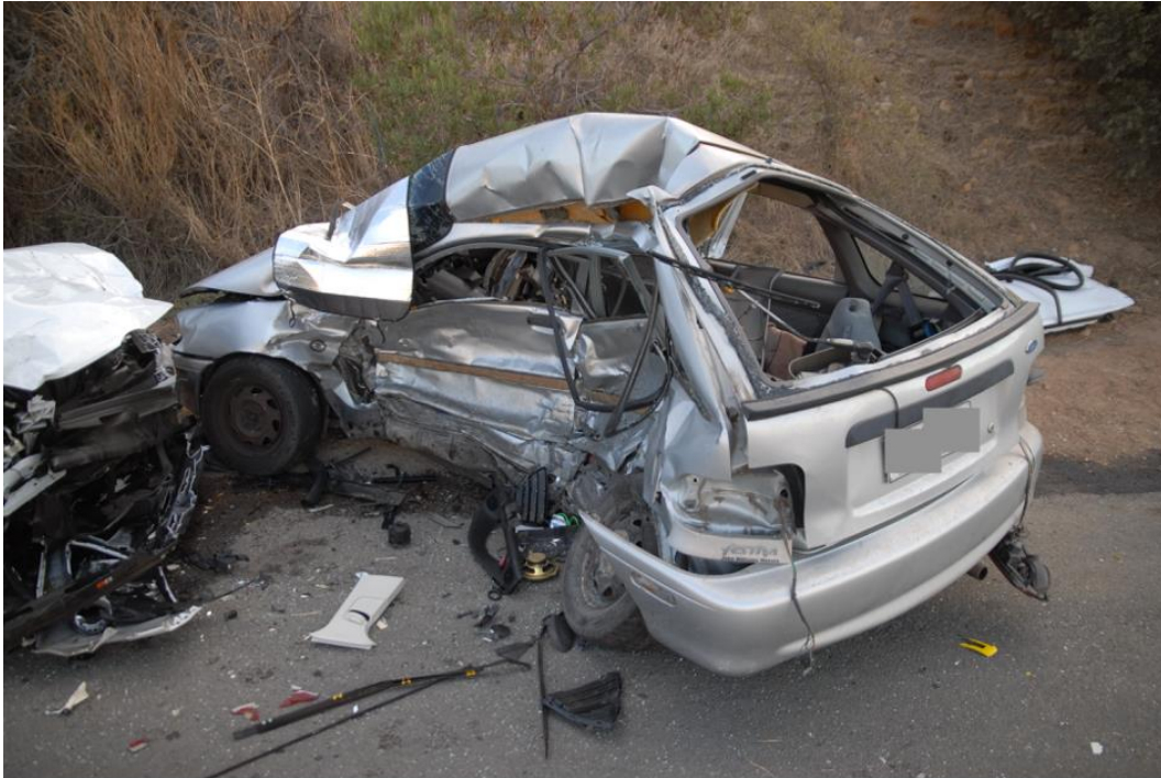
Figure 3.8 Typical side impact damage from loss of control type head on crash
