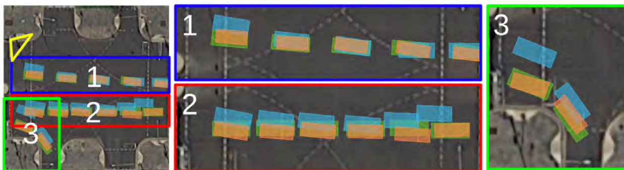
Figure 5: Detections of the same vehicles with the baseline model and the WIBAM model
