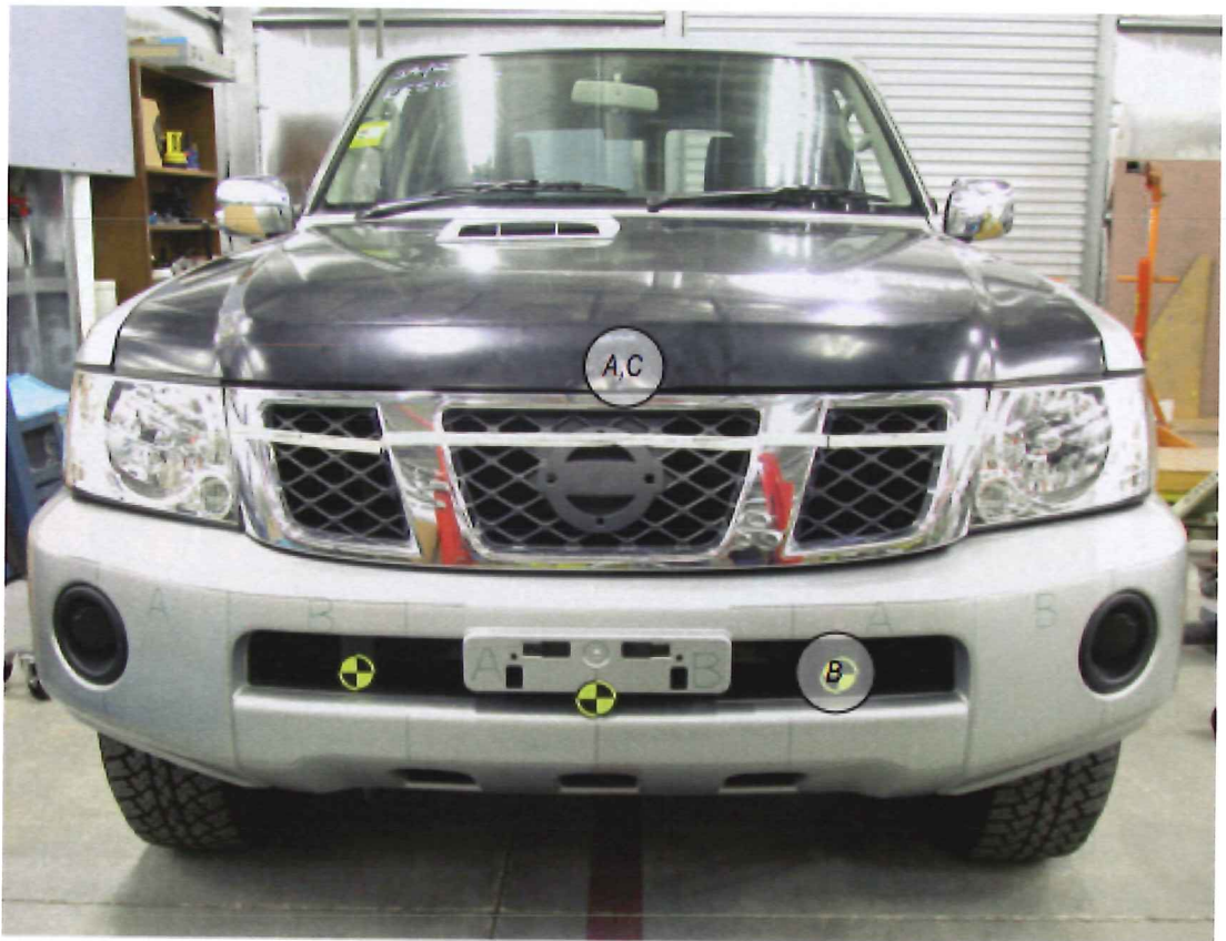
Figure 3.4 Nissan Patrol test locations. Letters correspond to test locations for Part A, B and C tests
