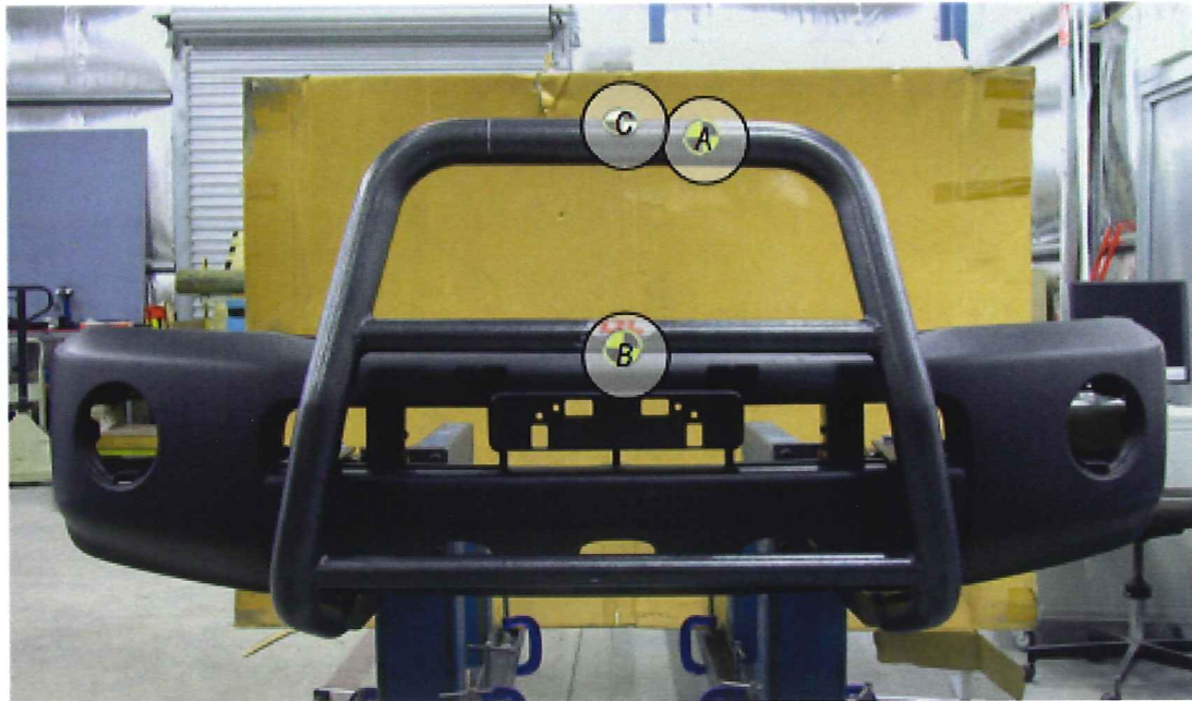
Figure 3.5 Nissan Patrol aftermarket alloy / aluminium nudge bar test locations. Letters correspond to test locations for Part A, B and C tests
