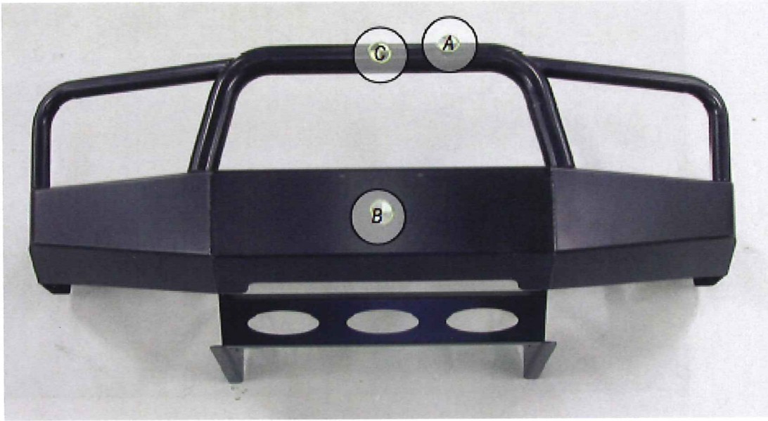
Figure 3.9 Ford Courier aftermarket steel bull bar test locations. Letters correspond to test locations for Part A, B and C tests
