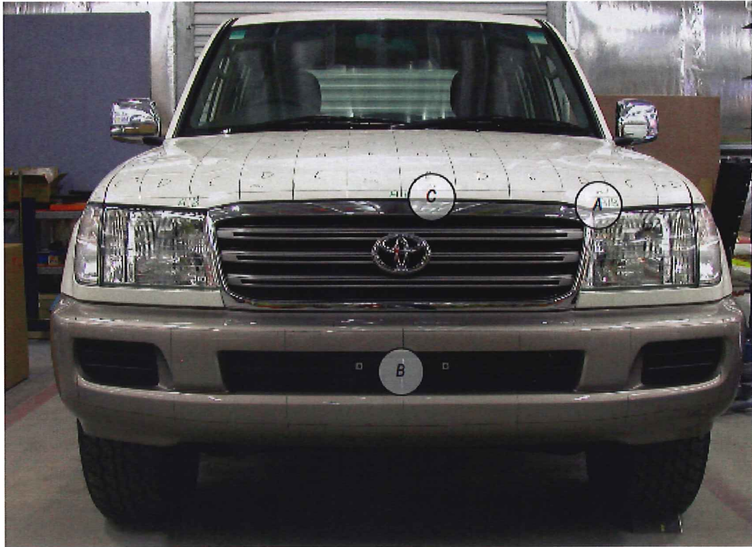
Figure 3.1 Toyota Landcruiser test locations. Letters correspond to test locations for Part A, B and C tests
