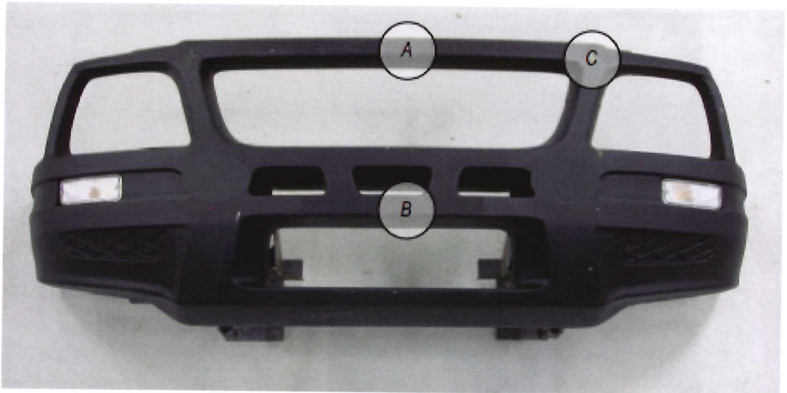
Figure 3.7 Nissan Patrol aftermarket polymer bull bar test locations. Letters correspond to test locations for Part A, B and C tests
