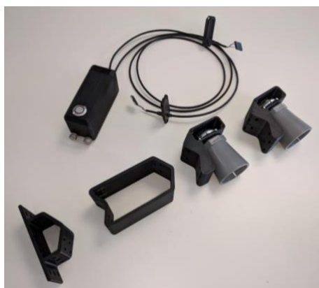
Figure 2.4 The PDMD-Mk2 main control box (top), ultrasonic mounting cases (right side), and mounting adaptors (lower left)
