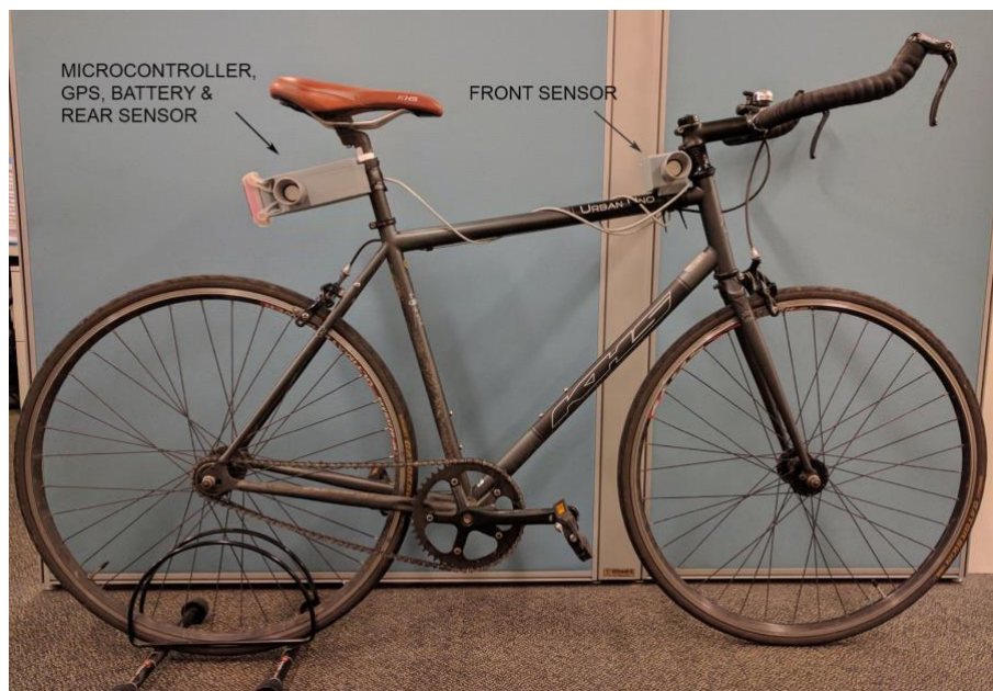
Figure 2.1 PDMD-Mk1 attached to a bicycle
