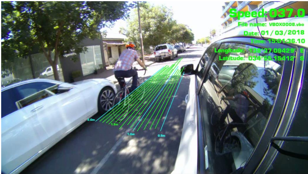
Figure 3.2 Video overlay system used to test the accuracy of the PDMD (In this image the cyclist is observed to be passed at a distance of approximately 1.4 metres)
