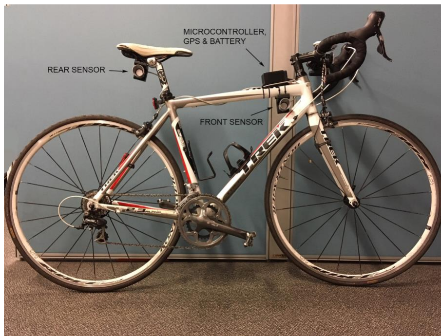
Figure 2.2 PDMD-Mk2 attached to a bicycle
