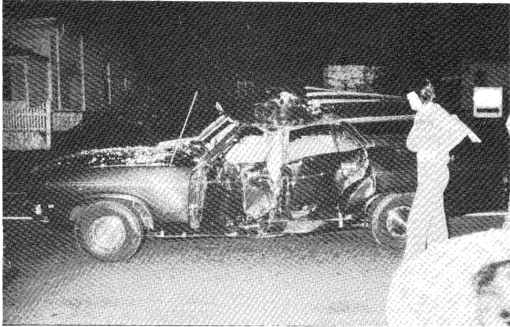
FIGURE 7: Car struck by motorcycle shown in Figure 8. Initial impact by front wheel of motorcycle was just behind the front edge of the front door. Damage to roof was largely due to impact from rider and passenger. See also Figure 9. Accident 042.
