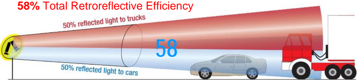
Figures 8B – Light return efficiency of Class 1X sheeting, 3M™ Diamond Grade™ DG3 Retroreflective Sheeting
