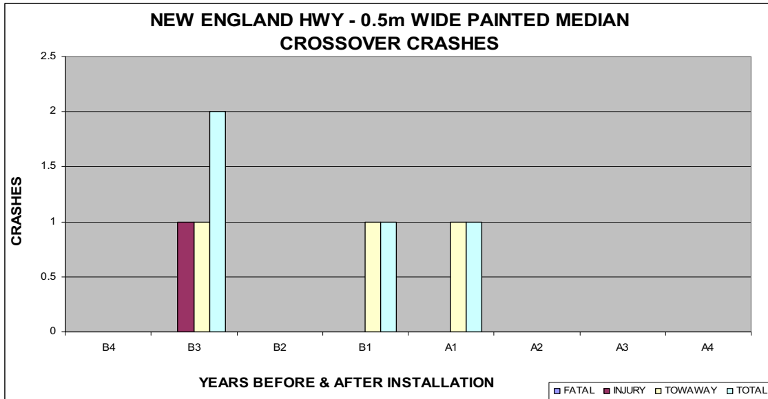
Figures 6 - New England Highway – 0.5m Wide Painted Median - Crossover Crashes
