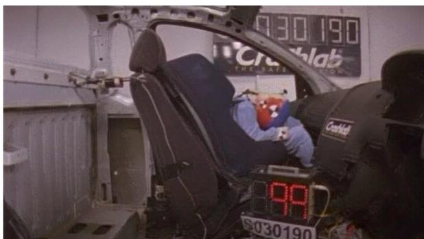
Figure 3. P-3 dummy in a forward facing CRS with no airbag deployment
