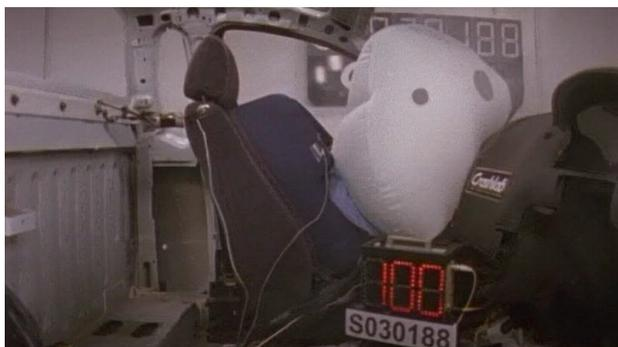
Figure 2. P-3 dummy in a forward facing CRS with airbag deployment
