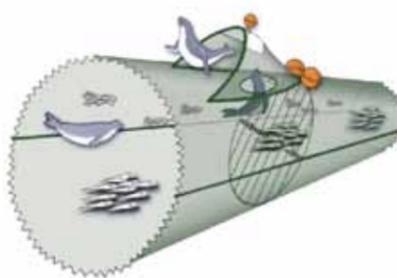
A photograph of a SLED (courtesy Dr Wendi Roe), and a diagram of the SLED, demonstrating the intended method of sea lion diversion (Tilzey and Wise, 2005)
