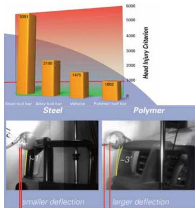
The difference: softer and lighter material deform more easily, cushioning the impact. This reduces the risk of injury in a collision.
