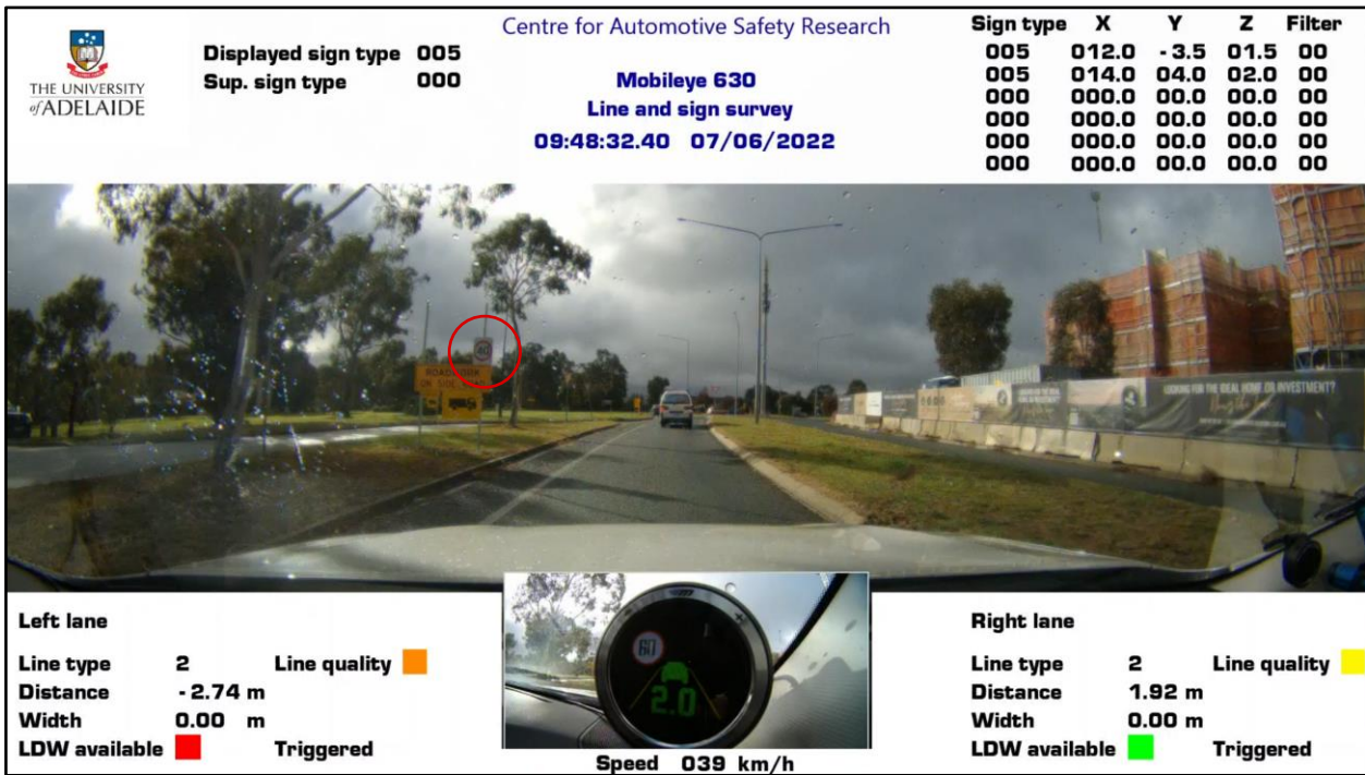
Figure B.1 Detected sign with a 40 km/h speed limit with a road segment tagged with a 60 km/h speed limit in the Open Street Map road network
