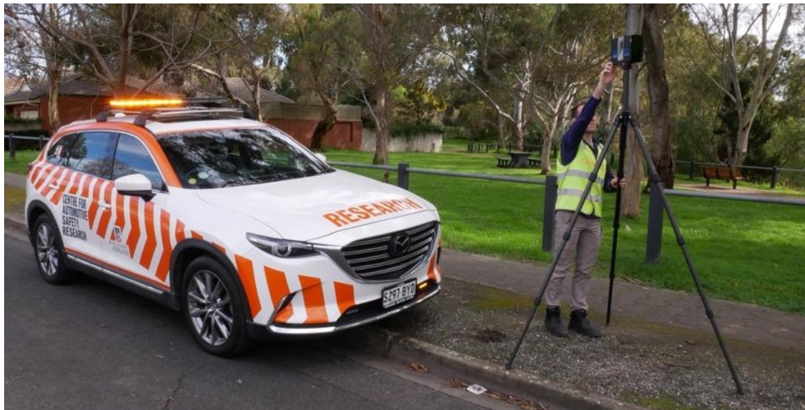
Figure 2.15 3D scanning equipment in-use at a crash scene
