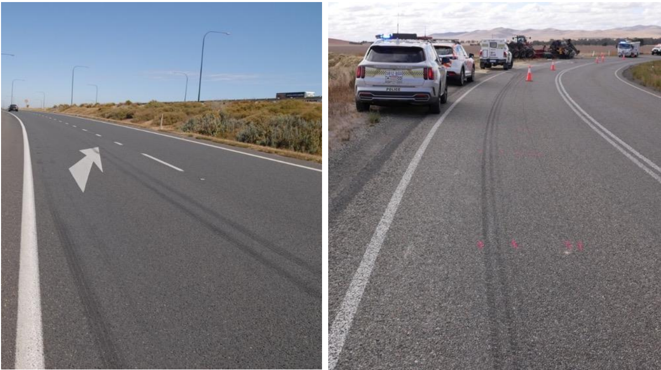
Figure 2.2 Examples of truck tyre marks from braking (left) and preceding a rollover (right)
