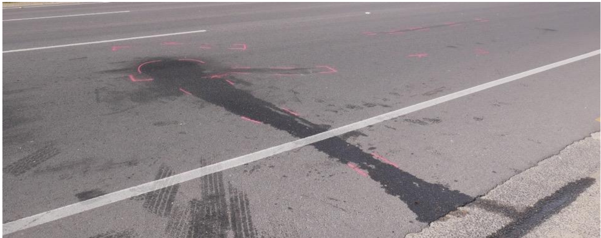
Figure 2.4 Example of fluid marks on a road left by a vehicle involved in a crash
