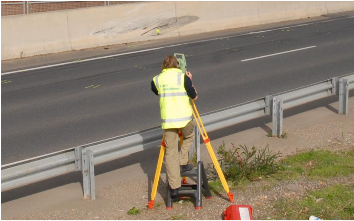
Figure 2.14 Total station surveying equipment in-use at a crash scene
