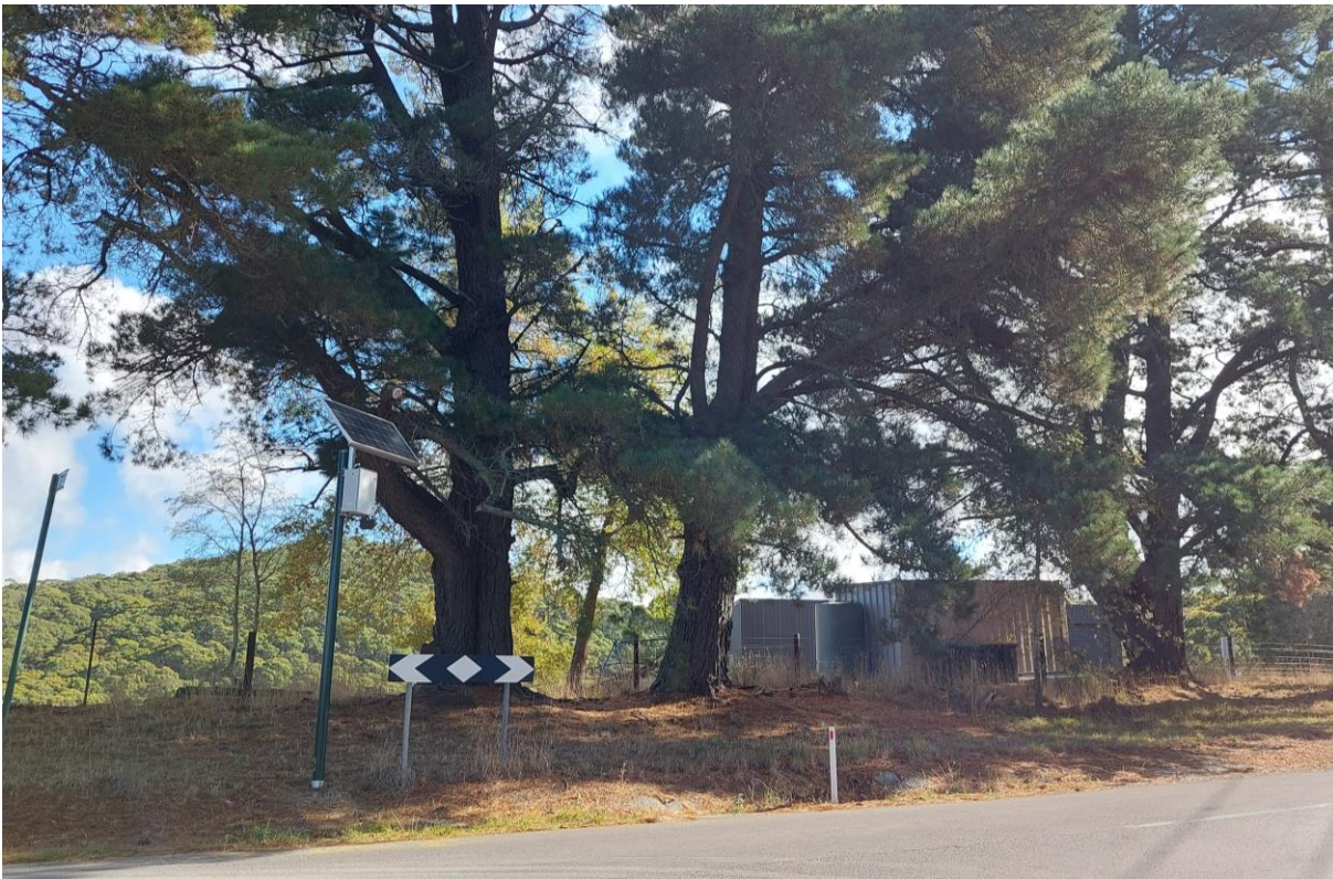
Figure 3.12 The minor road radar before it was moved, showing the density of foliage above the solar panel
