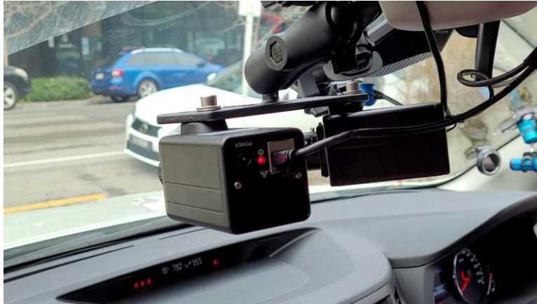
Figure 2.3 AeroRanger cameras mounted to windscreen of test vehicle
