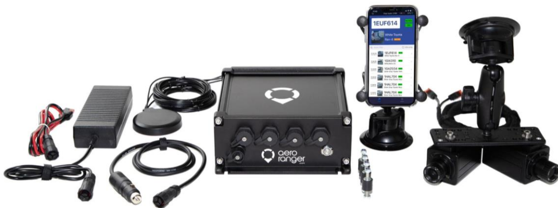
Figure 2.2 Components of AeroRanger ANPR system
