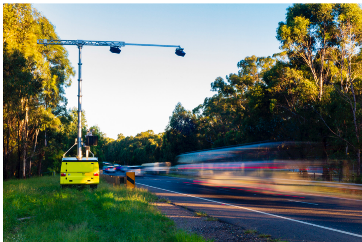
Figure 3.1 Acusensus Heads Up system deployed in mobile trailer configuration (source: acusensus.com)
