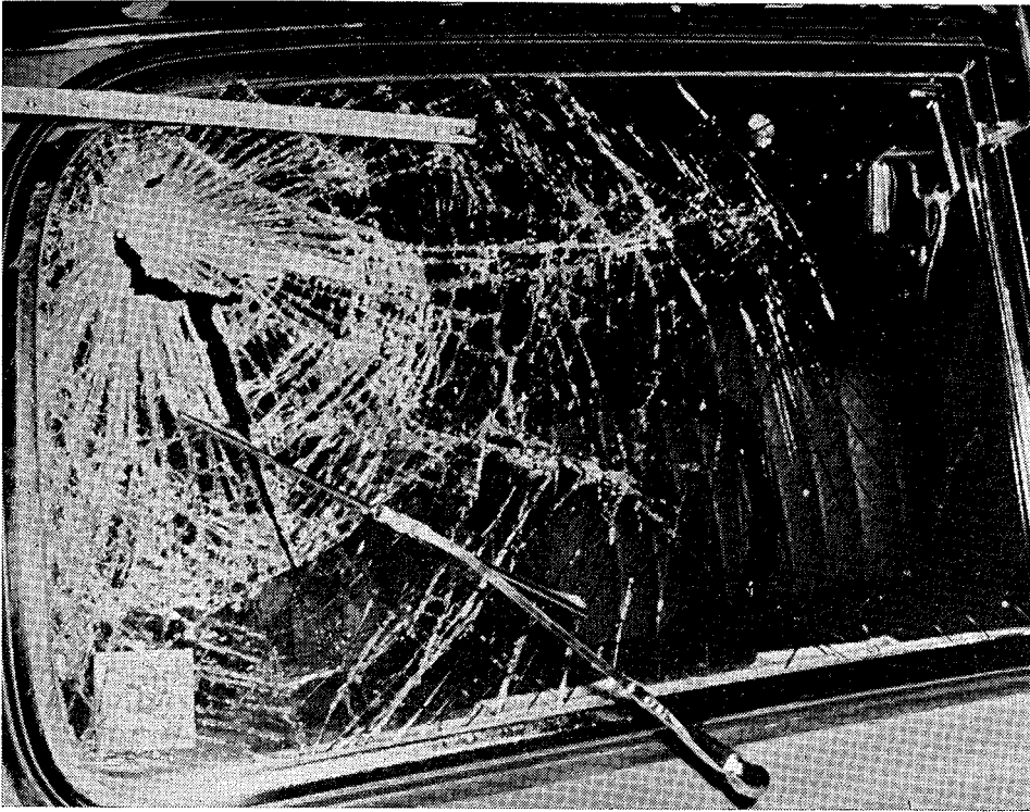
Fig. 11.8—Laminated glass windscreen not penetrated by occupant's head; minor lacerations of the face resulted
