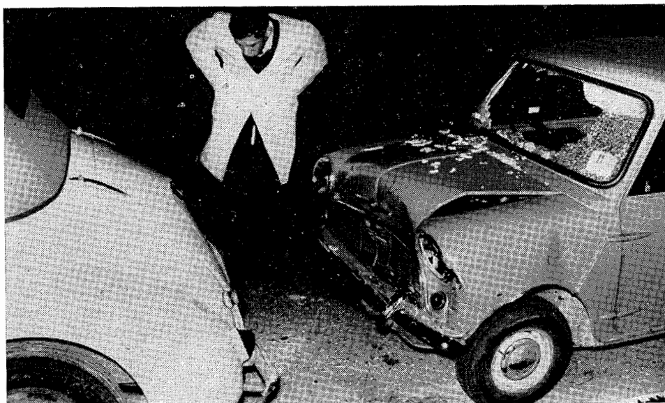
Fig. 11.21—Mini Minor struck stationary car. The driver, not wearing a seat belt, broke the windscreen with his head
