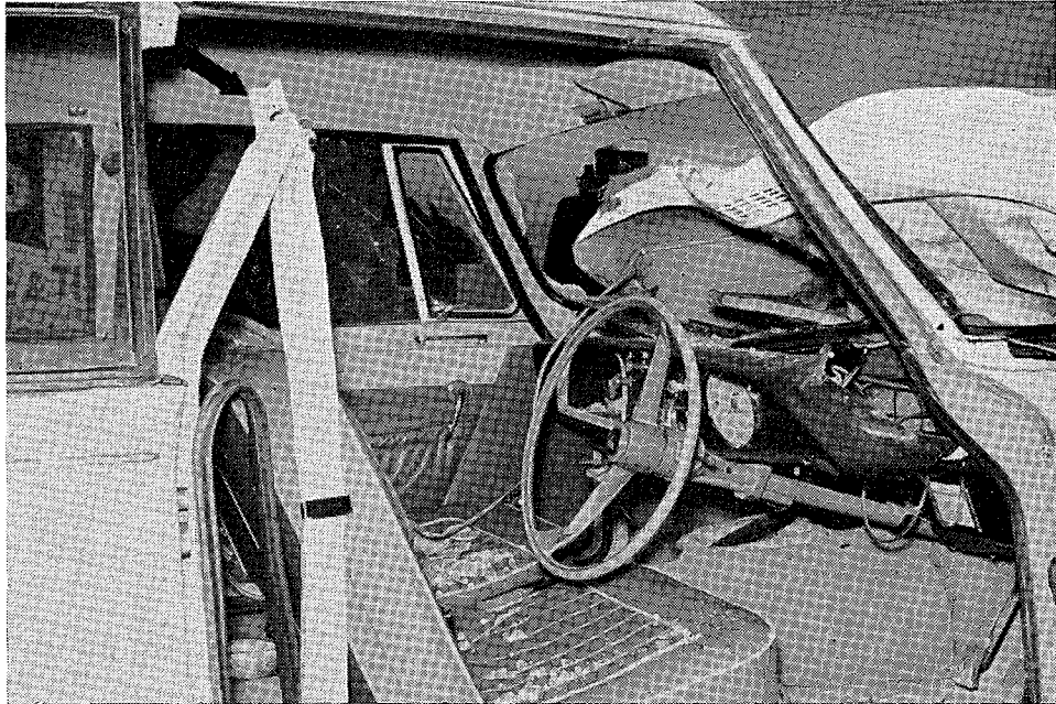
Fig. 9.33—Failure of seat belt mounting (arrow) on a 1960 Triumph Herald. Distortion of the mounting on the passenger's side is also indicated. This vehicle is also shown in Fig. 7.8
