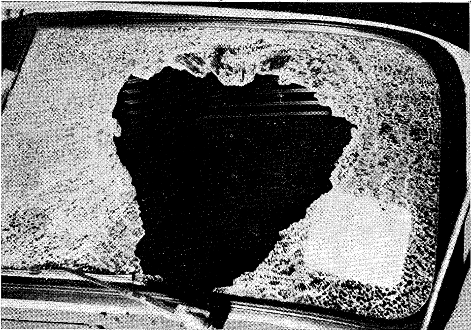
Fig. 11.6—Characteristic shape of hole in tempered glass windshield after impact by occupant's head
