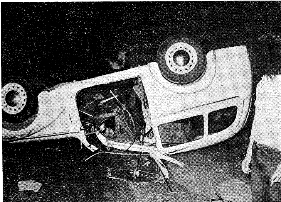
Fig. 8.23—This Skoda rolled over after swerving from one side to the other on a straight road
