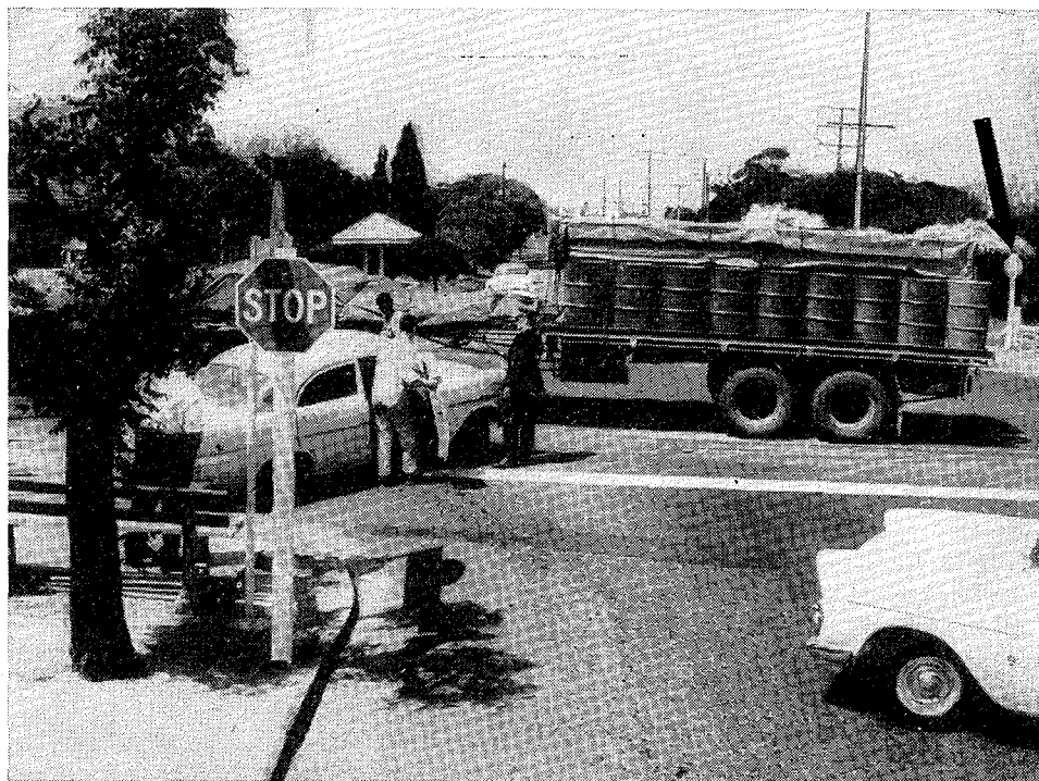
Fig. 10.16—Stop signs: this semi-trailer was unable to slow down sufficiently to avoid hitting the car which had moved off from the stop sign (arrow) on the far side
