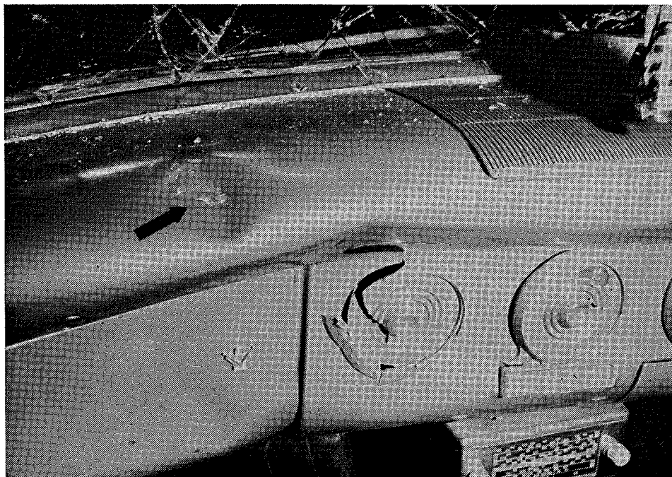
Fig. 11.18—Case 0046: frontal impact. Passenger's knee struck face of instrument panel, and his face and teeth struck top of instrument panel (arrow). Note teeth marks
