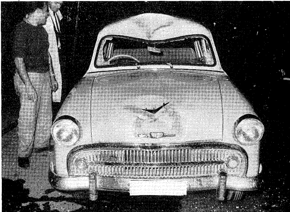
Fig. 5.13—Head-on collision between car and bicycle (dent in roof made by rider's head)
