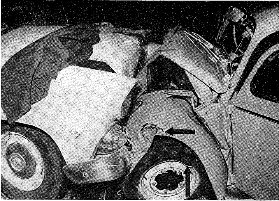
Fig. 8.6—Case 0046: arrows indicate the damage due to the initial collision between the Volkswagen and a Ford
