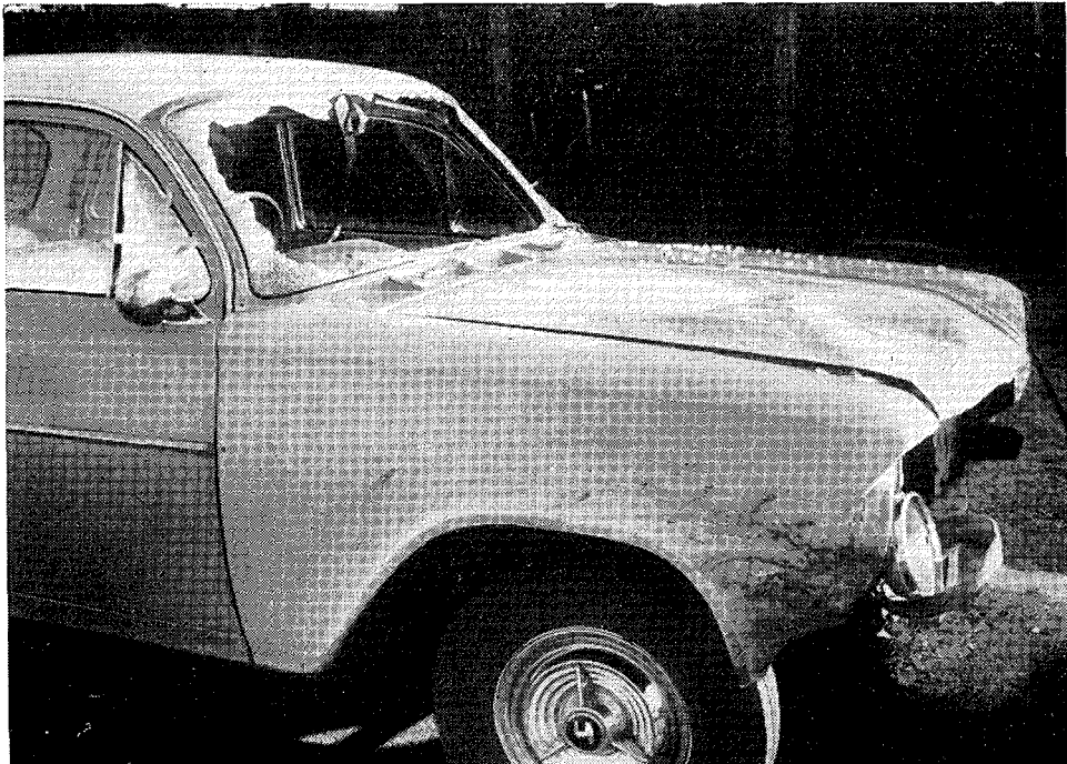
Fig. 5.7—Case 0367: rider of bicycle made dent in top of bonnet, broke the windscreen and slid along the roof (bumper and grille had been removed before the accident)
