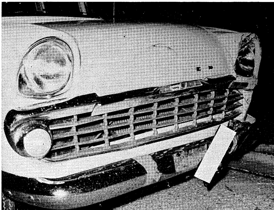
Fig. 9.12 —Note the relatively small amount of damage to this car. The struck car (see Fig. 9.11 ) was spun anti-clockwise by the impact and rolled over
