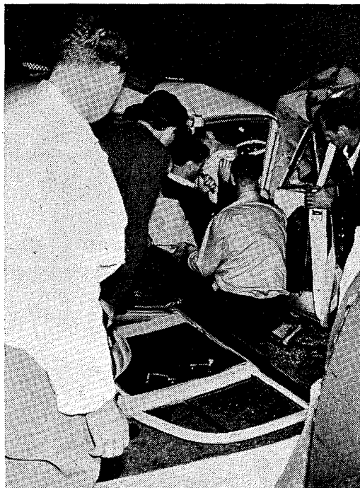
Fig. 9.22 — Driver trapped in an FX Holden by the front seat, which moved forward in the collision
