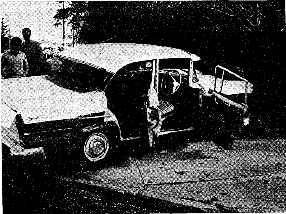
Fig. 9.34—1960 Vauxhall Victor, struck on the right side by another car at an intersection. Both doors on the right side were sprung open
