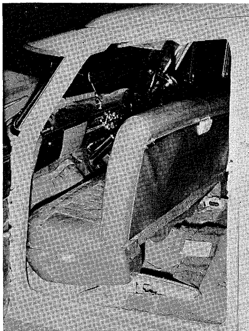
Fig. 9.24 — Front seat completely off adjustment runners, 1953 Ford Customline (also shown in Fig. 9.16)
