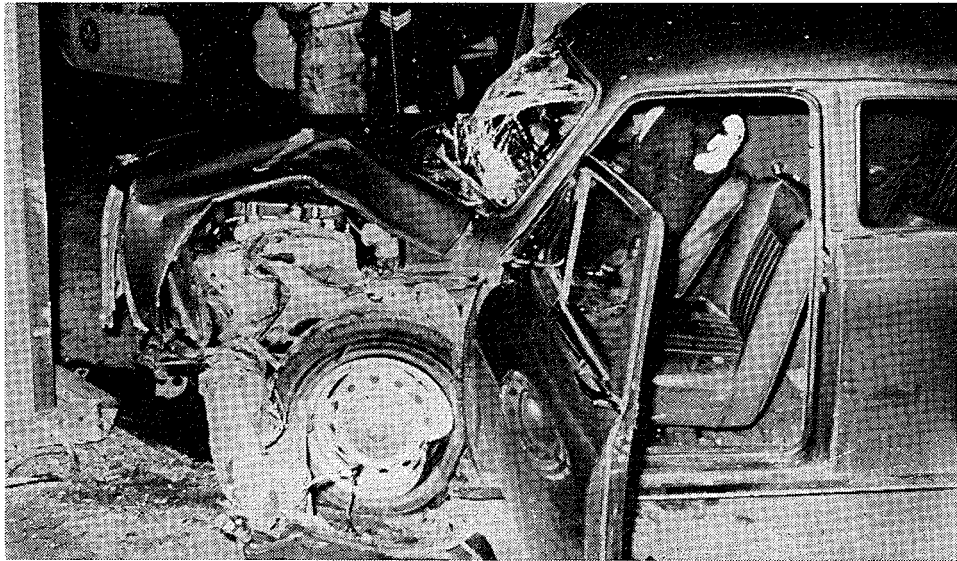
Fig. 8.22—1954 M.G. Magnette after colliding with the utility pole shown (see also Fig. 9.29, 11.7 and 11.17)
