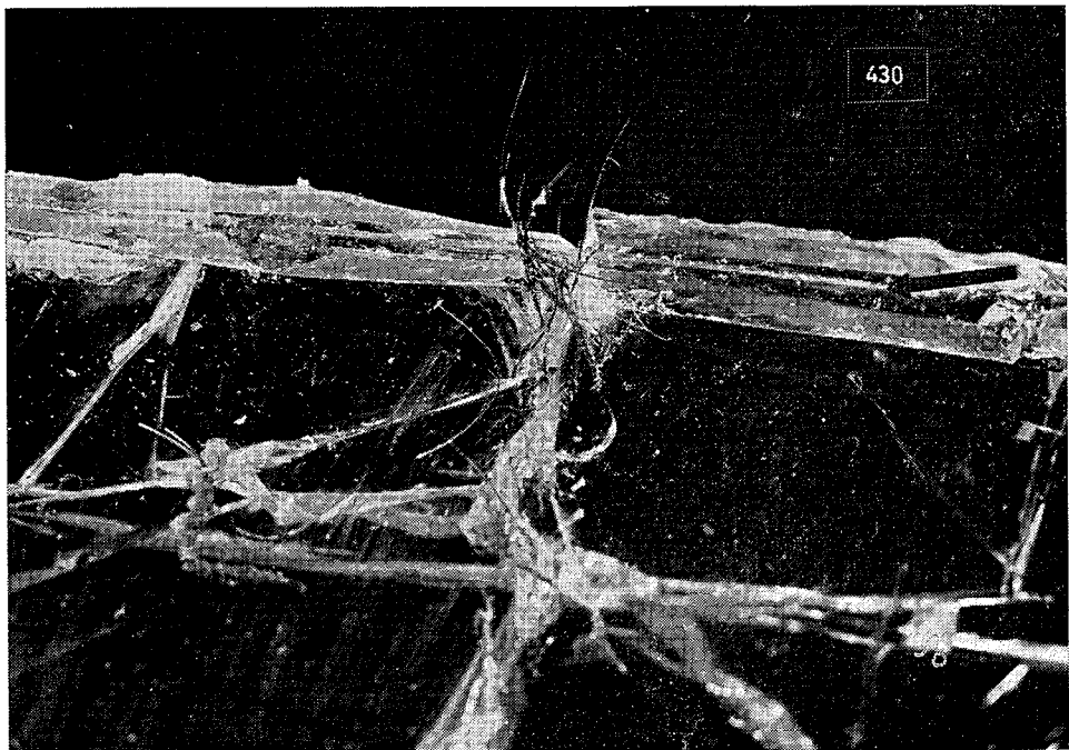
Fig. 9.29 — Laminated glass windscreen of a 1954 MG Magnette saloon, broken by the passenger's head; note hairs caught on sharp edges. Arrow indicates the interlayer between the two sheets of glass
