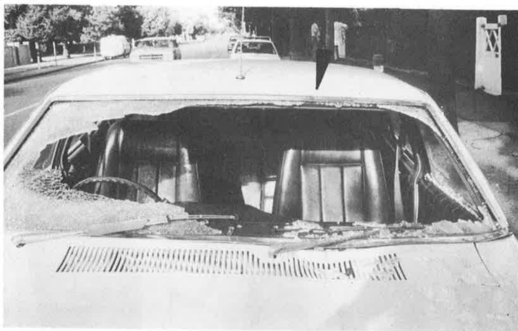
FIGURE 8: Damage resulting from collision with cyclist. Note small dent in trim above windscreen (arrowed). Accident 250.
